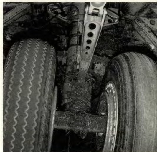
The B-47 settled short of the runway. The left outrigger struck the soft ground causing the main left gear to roll in the dirt for 50 feet. The left outrigger doors contacted the runway during the last 300 feet of landing roll as the pods bend downward. Approach too low, flat.
