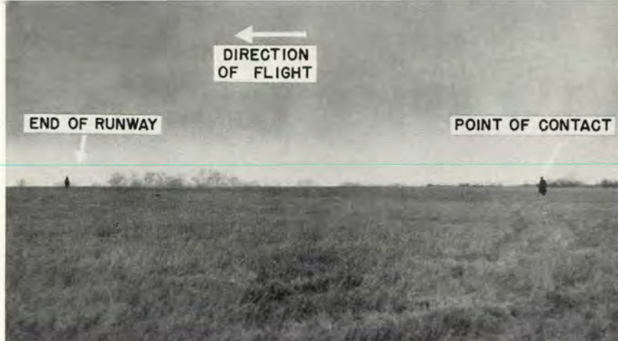
The B-47 settled short of the runway. The left outrigger struck the soft ground causing the main left gear to roll in the dirt for 50 feet. The left outrigger doors contacted the runway during the last 300 feet of landing roll as the pods bend downward. Approach too low, flat.
