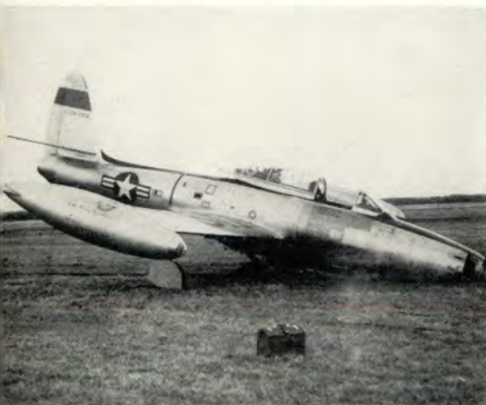
Pilot misjudged distance. Landed 100 feet short. Nose gear plowed up sod, then folded.
