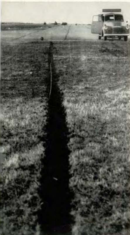
Pilot misjudged distance. Landed 100 feet short. Nose gear plowed up sod, then folded.
