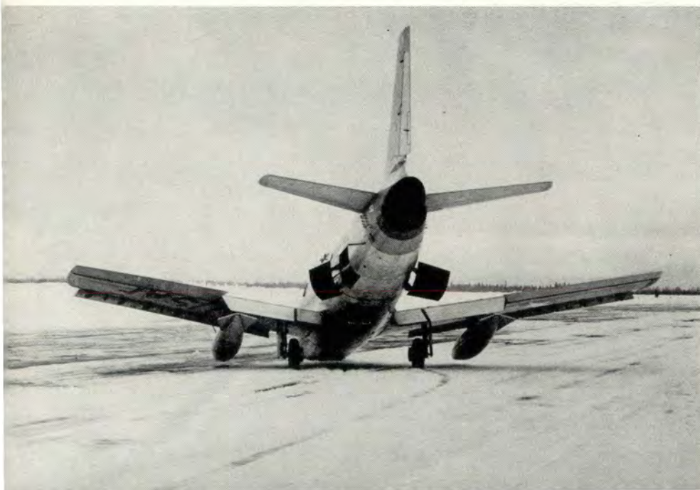
Too low on final. Above, main gear touched first in snow, forcing nose gear down. Slid 1500 ft.
