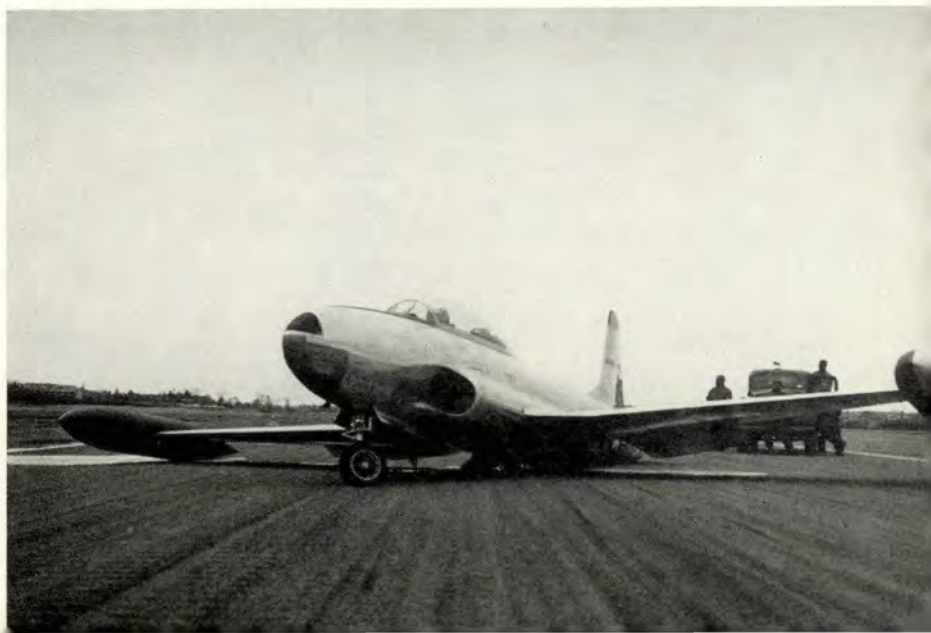
Pilot failed to maintain sufficient altitude and airspeed to compensate for gusty wind conditions. T-33 struck wooden warning fence, above, bounced and slid to stop.
